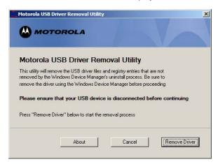
7 Click Remove Driver. A progress bar indicates that the driver is being removed.
